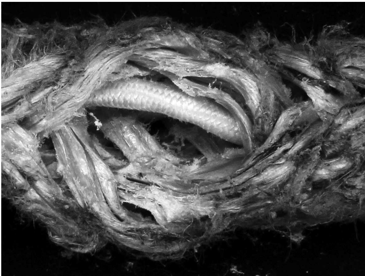
Figure 30-2.8.2-3 Damage Inside the Rope
