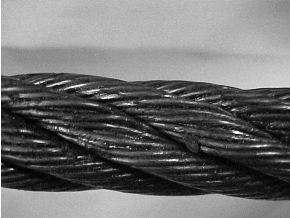
Figure 30-1.8.2-4 Distortion of Rope Structure — Crushing
