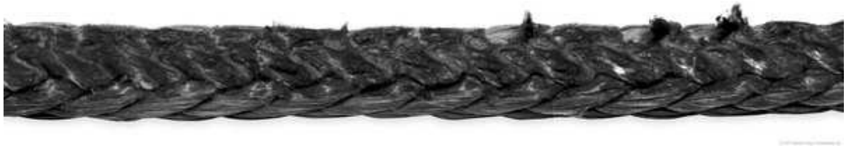
Figure 30-2.8.2-5 Melt Damage Due to Heat
