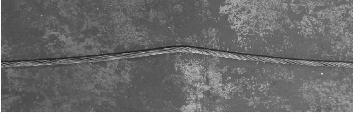
Figure 30-1.8.2-2 Distortion of Rope Structure — Dogleg
