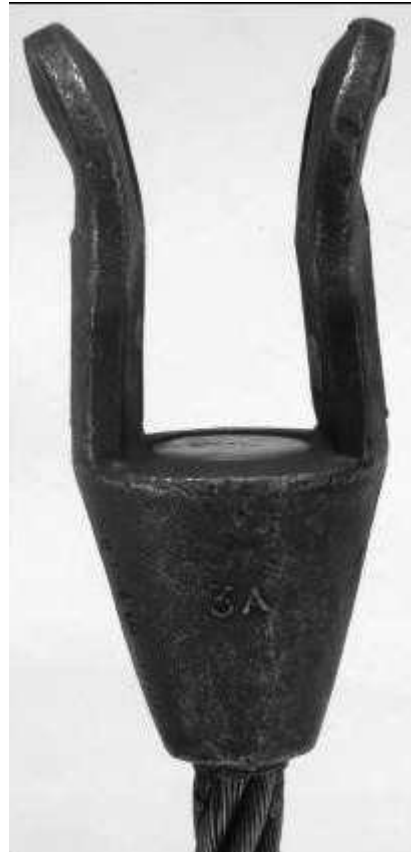
Figure 30-1.8.2-9 Damaged End Terminations
